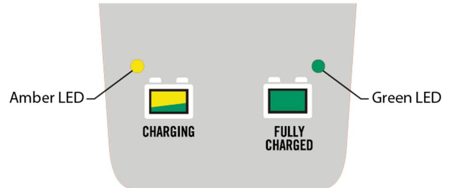
When AC power is first applied to the charger all of the LEDs will illuminate for two to three seconds before starting the charge sequence listed below.
