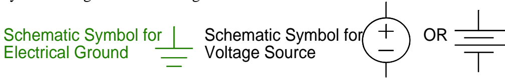
Figure 5 Schematic Symbols: GND & Voltage Source
